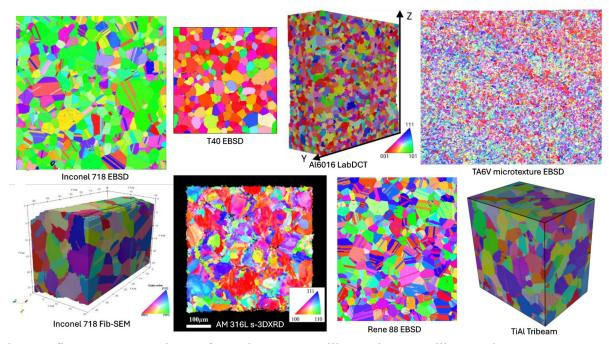
Above figure: examples of various metallic polycrystalline microstructures, including steel, aluminium, titanium and nickel based alloys; these microstructure were characterized by electron of X-ray diffraction, in 2D (surface) or 3D (tomography). All images are depicted using inverse pole figure coloring related to the crystal orientation.
